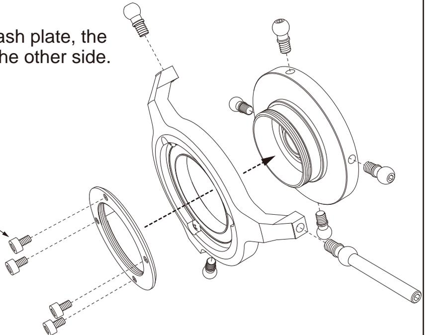
Use the hand tool on the screws, turn clockwise to tighten, counter-clock-wise to un-tighten.
