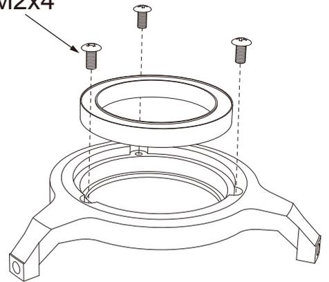
Insert the M2x3 Screws into the swash plate, the screw threads should not protrude the other side.
