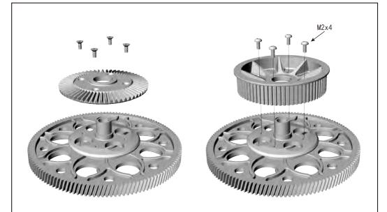
Disassemble the bevel gear and replace with the belt gear as the illustration in next page.
