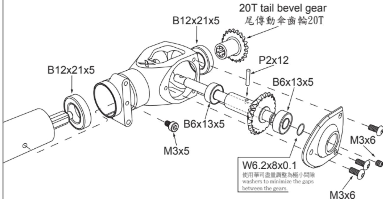
Insert the 20T tail bevel gear, then fix the gear case cap.
